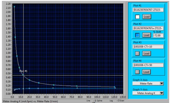
But performance becomes worse as the viscosity increases to 50 mm<sup>2</sup>/s (white curve). Below 75% of the range the deviations rise above 2% and up to 34%.
